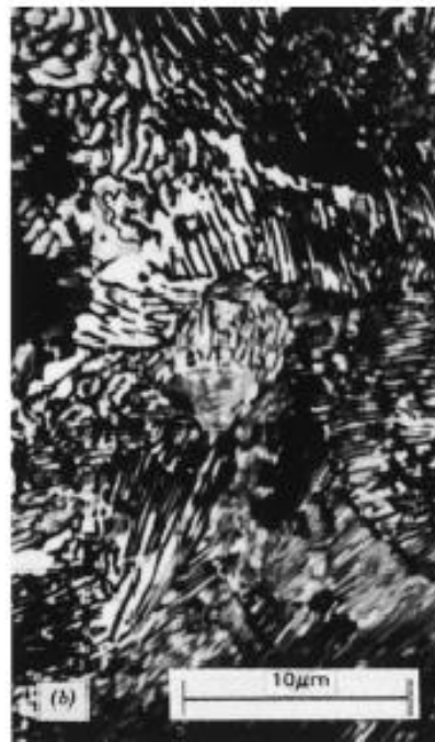
FIGURE 11.6 Photomicrographs of (a) coarse pearlite and (b) fine pearlite. 3000 \times . (From K. M. Ralls, et al., An Introduction to Materials Science and Engineering , p. 361. Copyright \copyright 1976 by John Wiley & Sons, New York. Reprinted by permission of John Wiley & Sons, Inc.)
