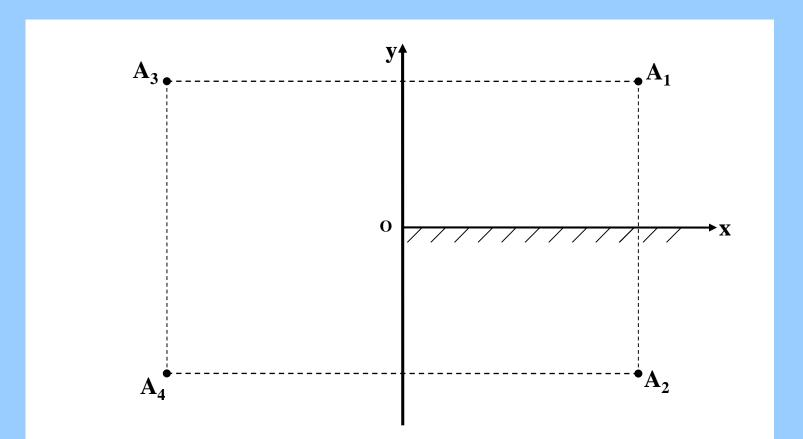
For an exact solution to exist, the following conditions should hold: a) The number of image wells should be finite. b) Their kind (pumping or inhecting) should be uniquely defined and c) Image wells should not be placed inside the real flow field.
