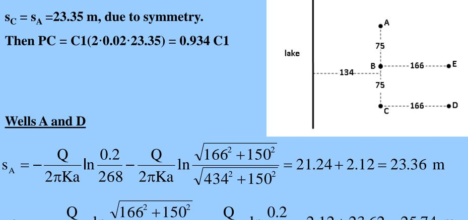
$s_{\rm D} = -\frac{Q}{2\pi Ka} \ln \frac{\sqrt{166^2 + 150^2}}{\sqrt{434^2 + 150^2}} - \frac{Q}{2\pi Ka} \ln \frac{0.2}{600} = 2.12 + 23.62 = 25.74 \text{ m}$
